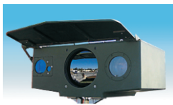
Long-range thermovision and LLLTV cameras Eye-safe laser rangefinder
