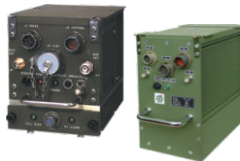
Interrogator and Cryptographic Computer MARKXII mode 4, NSM, upgrade mode 5, mode S
